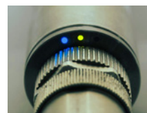
The blue LED indicates falling thermal intensity
