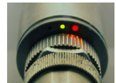
The red LED indicates rising thermal intensity
