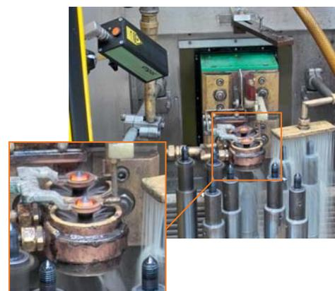
Pic. 5: Pusher feed hardening of a special screw.
