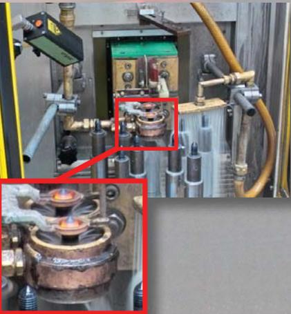
Pusher feed hardening of a special screw
