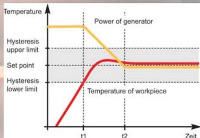
*Automatic temperature control using a proportional controller*
