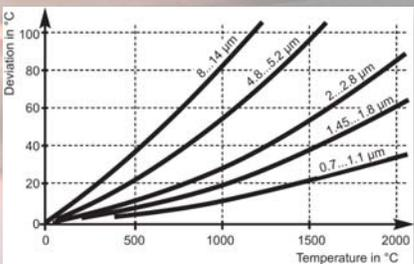
Measurement errors caused by incorrect selection of pyrometers. To demonstrate the temperature reading errors, the emissivity was incorrectly adjusted by 10%
