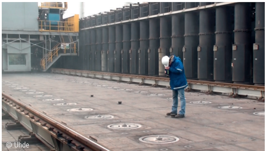
Measurement of coking oven temperatures from the oven roof through the inspection hole
