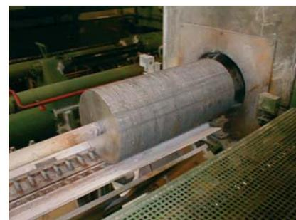
Pic. 7: Temperature control of preheated billet before extrusion.
